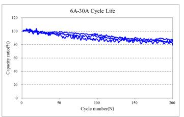
Charge : CC-CV 1.25A to 4.2V, 100mA cut-off at 25±2°C
