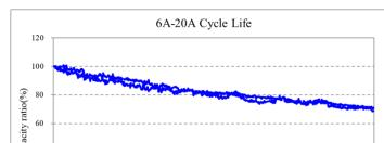
Charge : CC-CV 6A to 4.2V, 100mA cut-off at 25±2°C Discharge : CC 30A to 2.5V&75°C cut-off at 25±2°C
